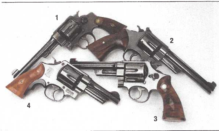
Four double-action Smith & Wesson revolvers used during testing include the (1) Second Model Hand Ejector .44 Special, (2) Model 20 .38 Special, (3) Pre-Model 27 .357 Magnum and a (4) Model 22 .45 Auto-Rim.
