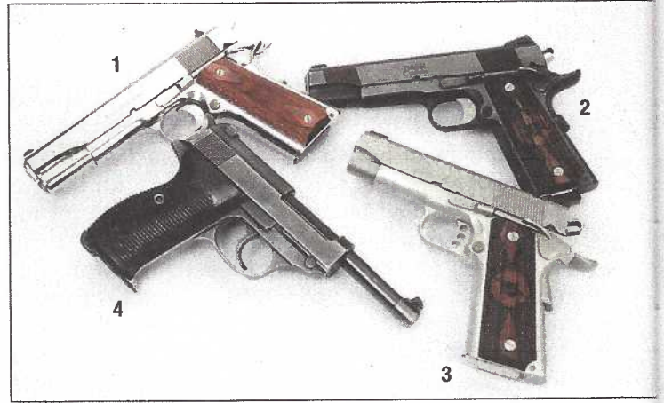
The four autoloading pistols used to test bullets include the (1) Colt Model 1911 El Centurion, (2) Les Baer Model 1911, Thunder Ranch Special .45 Auto, (3) Kimber Pro-Carry .40 S&W and a (4) German (Mauser) P38 9mm.
