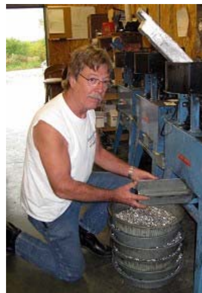
BRAD ALPERT removes bullets from one of the four casting machines in his shop in rural Kingsville, where the enterprise turns out 100,000 bullets on an average day. SUE STERLING/Star-Journal photos
