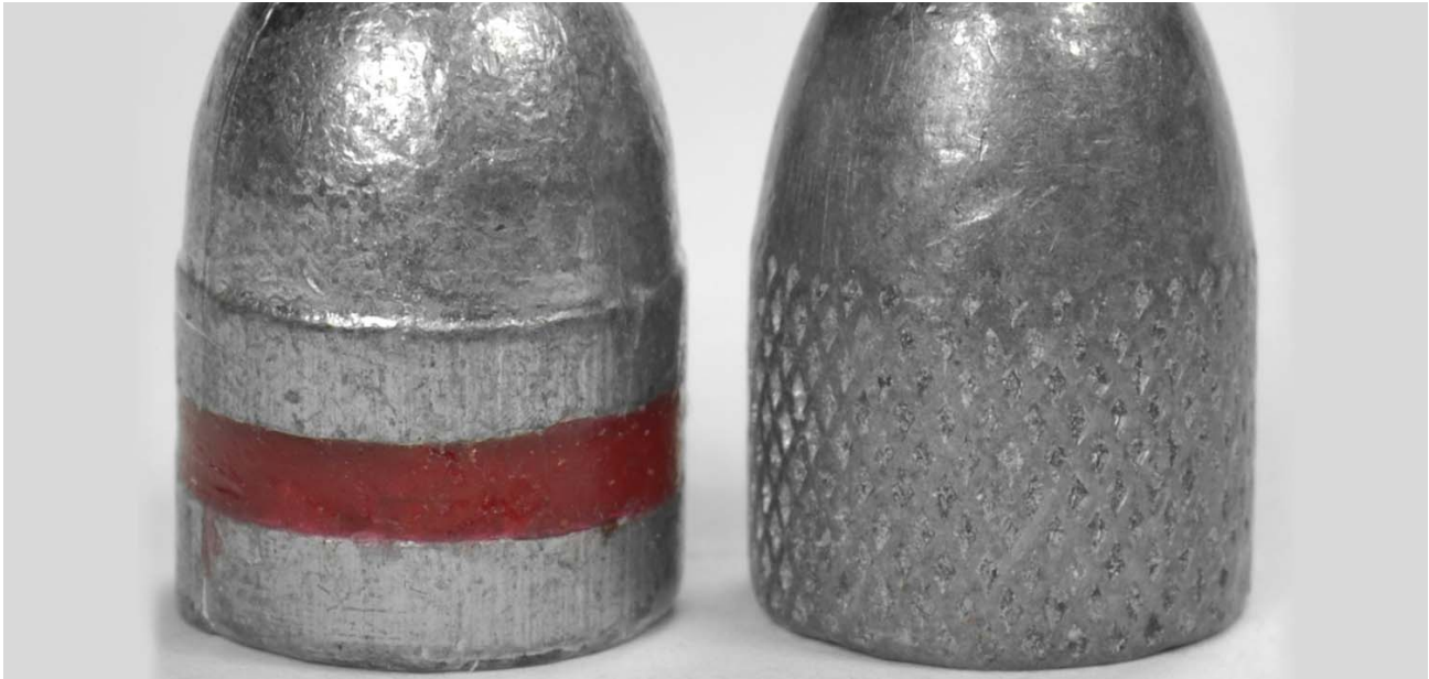
Figure 1. Traditional lead bullets are cast (left) or swaged (right). Both are lubed with a waxy lube.
